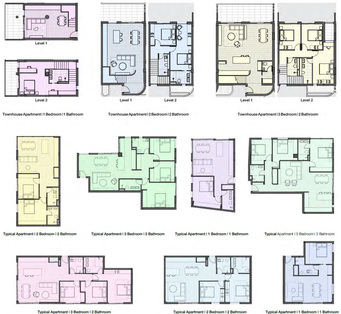
Figure 6: Typical Split Level Apartment and Standard Apartment Layouts
