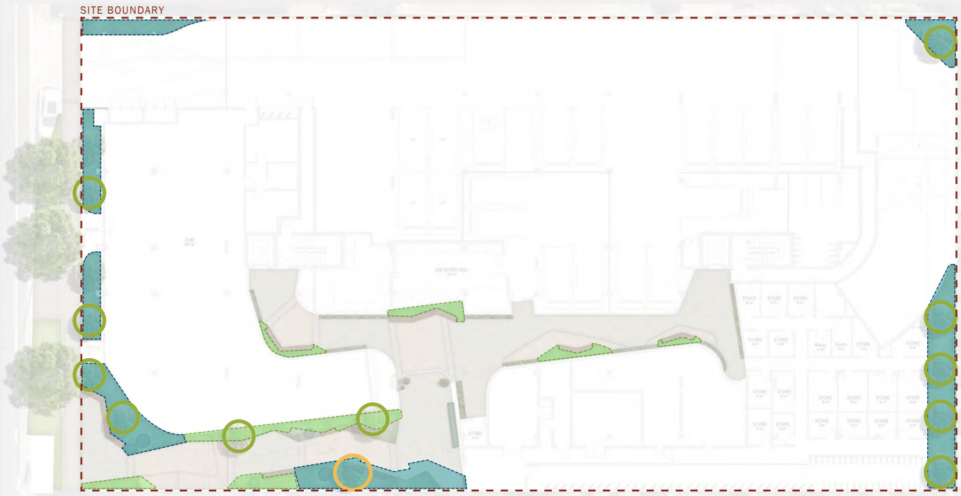
FIGURE 1. GROUND FLOOR DEEP SOIL REQUIREMENTS (AS PER SPP 7.3 DESIGN GUIDELINES)
