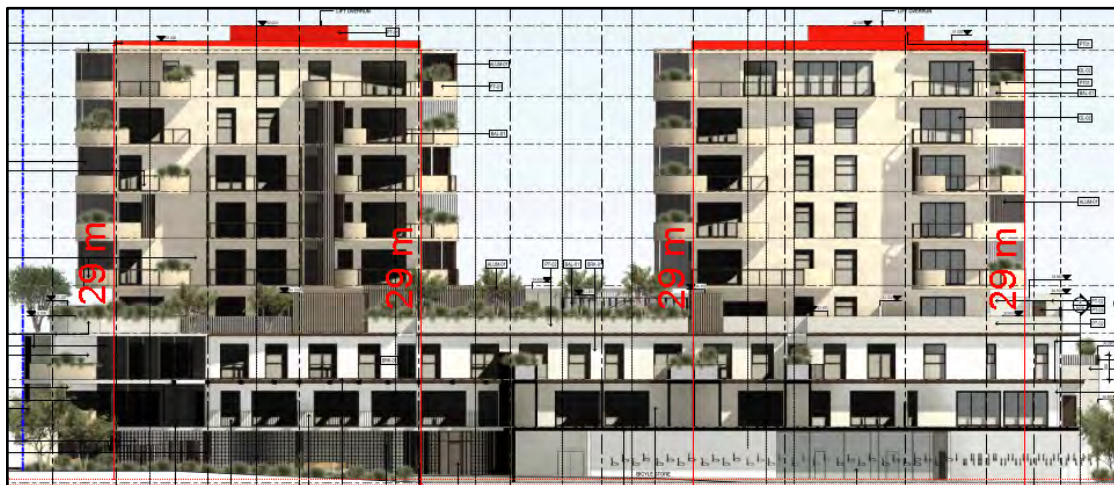
Figure 4 Extract from Planner Assessment of compliant building height (29m) marked in red - eastern elevation.
