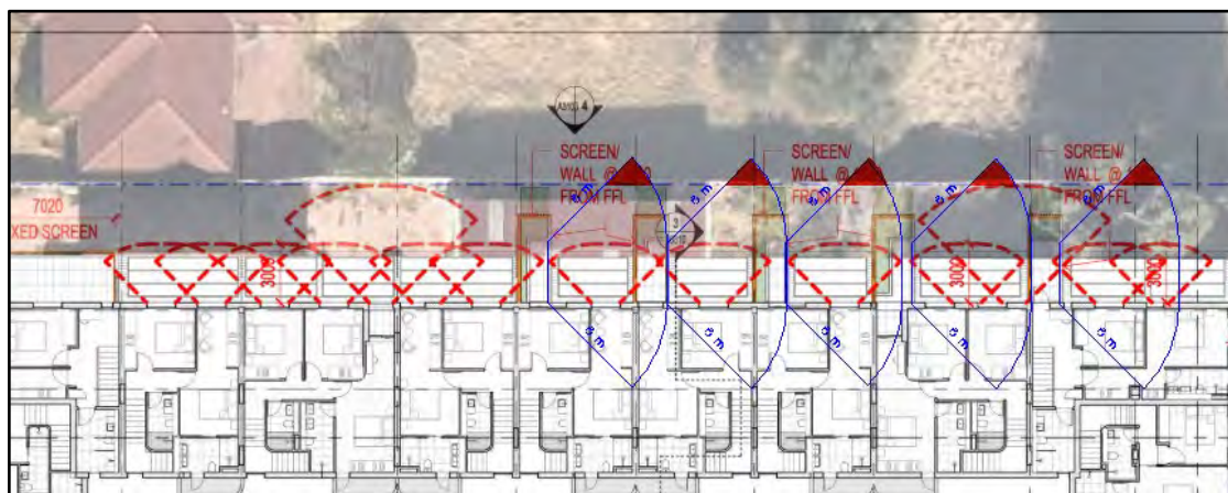
Figure 8 Extract of Planners Assessment Showing Overlooking from Level 3 Western Balconies into Lot 42, House Number 22 Brighton Road Scarborough.
