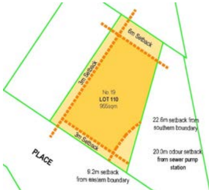
Figure 1: Built Form Envelope
