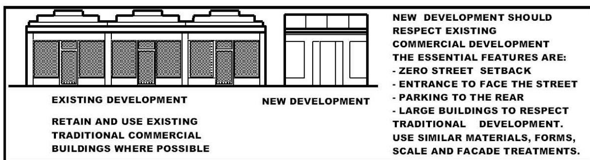
Figure 34 – Example of New and Existing Development
