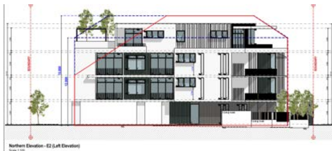
Figure 3: Extract from Architectural Plans with City's mark ups showing proposed building in relation to permitted wall and roof height (shown in red)
