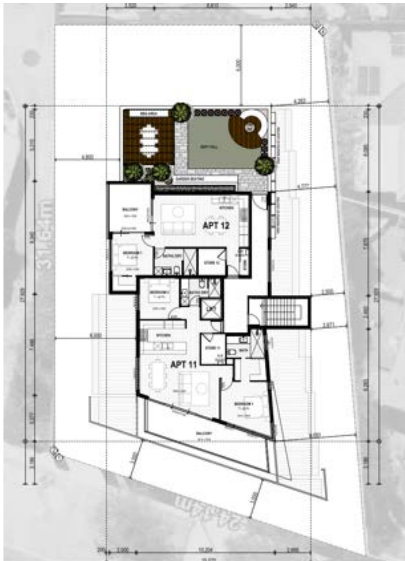
Figure 6: Extract from the Architectural third floor plan detailing extent of reduced setback to the southern lot boundary
