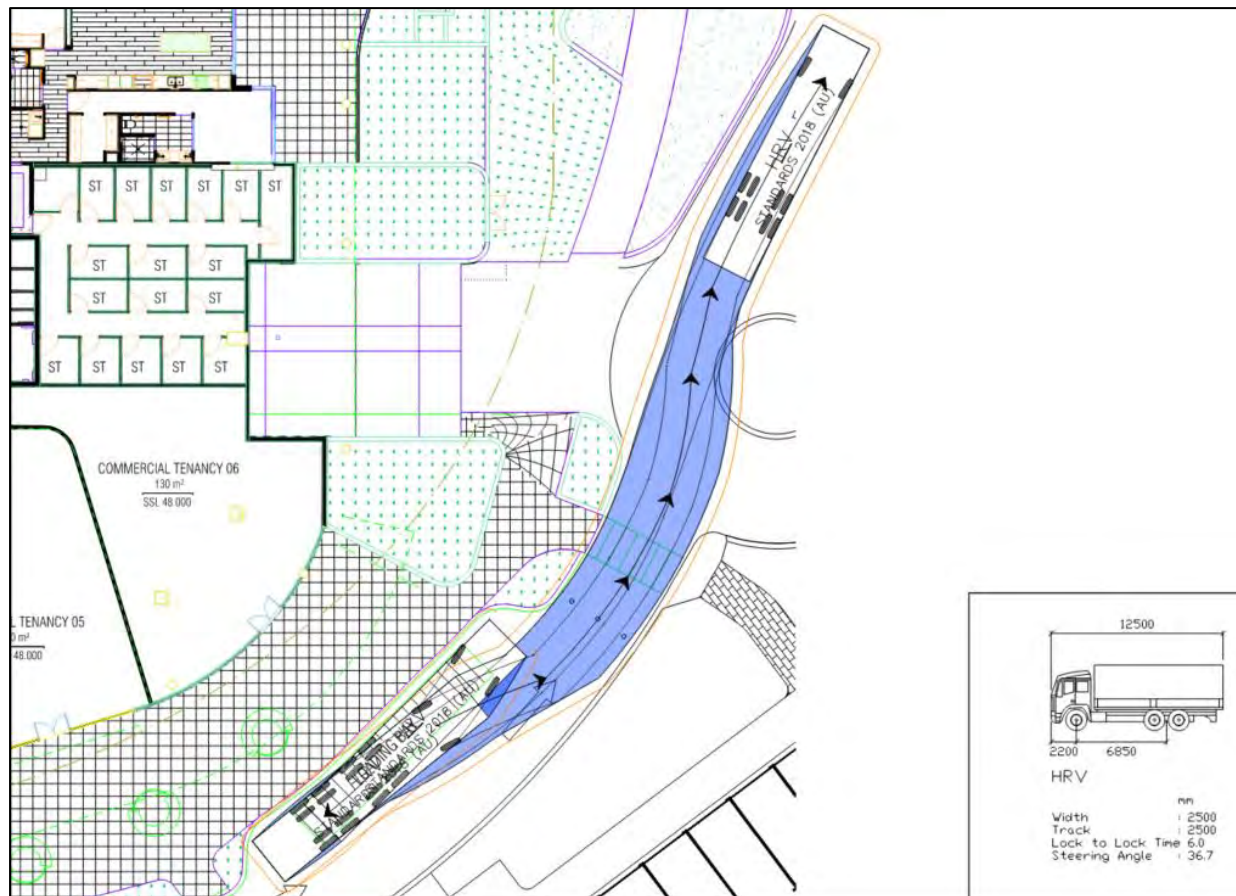
Figure 4 HRV Design Vehicle Exiting Loading Bay
