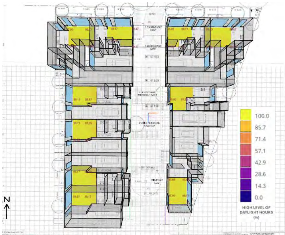
Figure 4: Daylighting for Ground Floor
