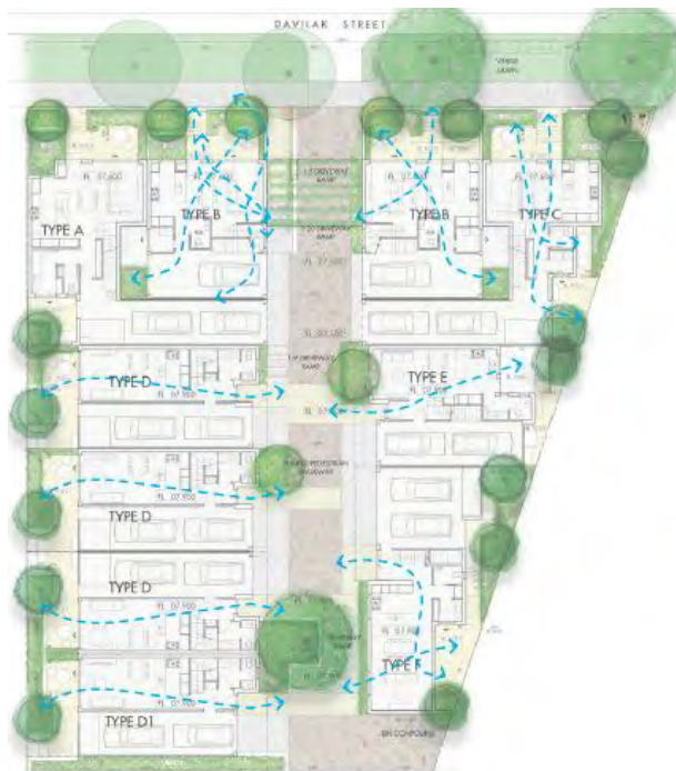
VENTILATION DIAGRAMS - GROUND FLOOR
