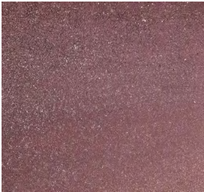
RED OXIDE ASPHALT - DRIVEWAYS/CARPARK
