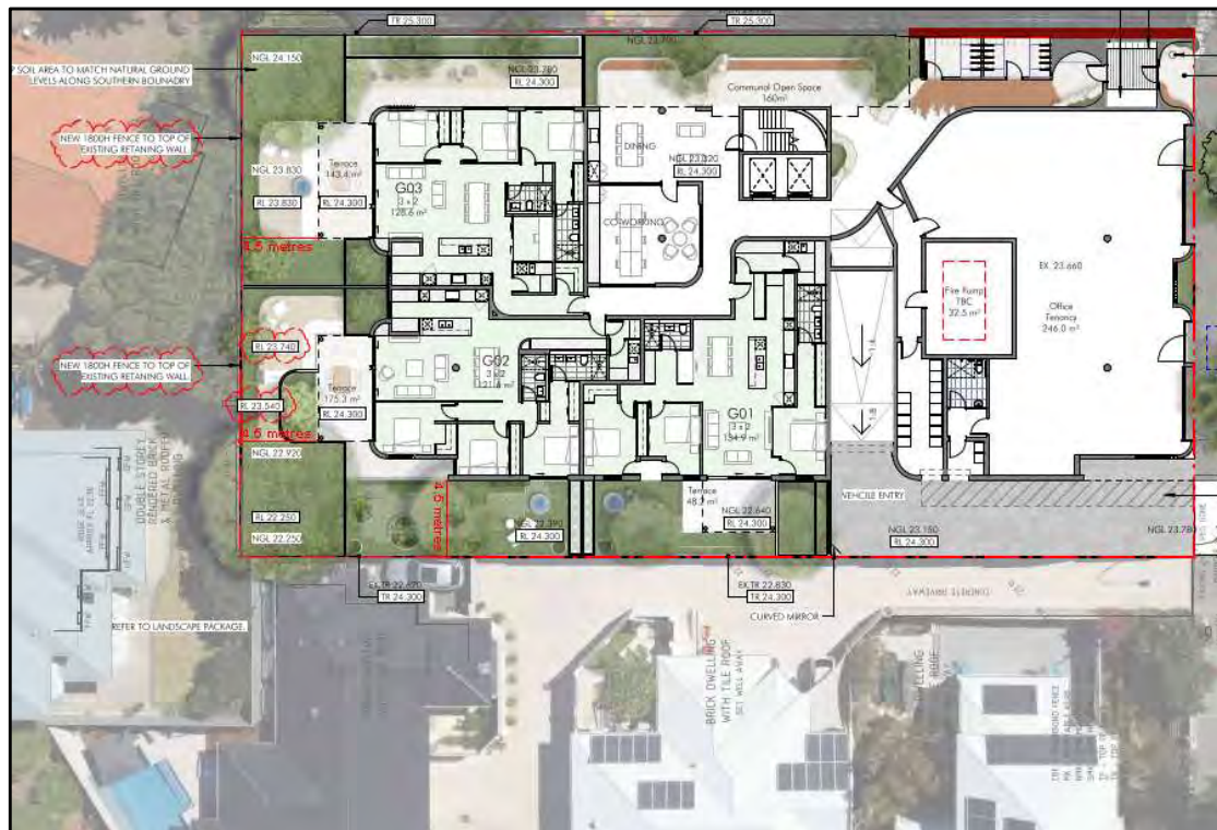
Figure 8 – Overlay showing the setbacks of the development to the southern and western boundaries.
