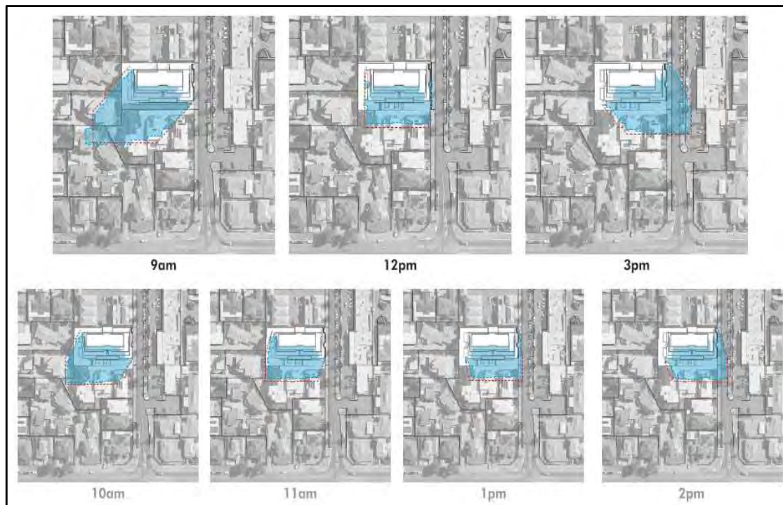
Figure 12 - Applicant's Winter Solstice Solar showing access to southern property solar PV panels. Red annotations demonstrating a minimum of solar access of 5 hours and burgundy demonstrating a minimum of 6 hours.
