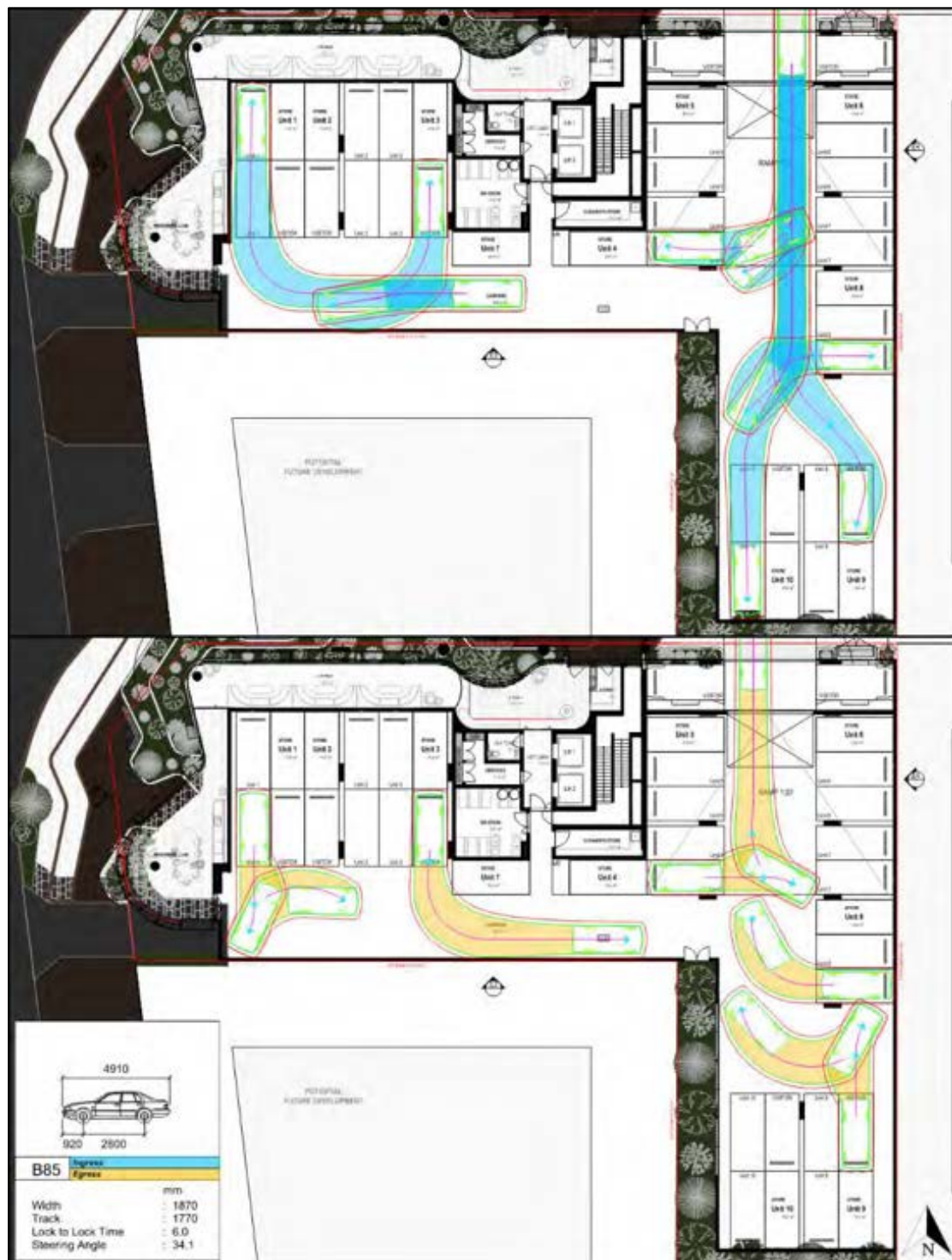
Figure 5-6 Swept Paths – Ground Floor Parking Area (gated area)
