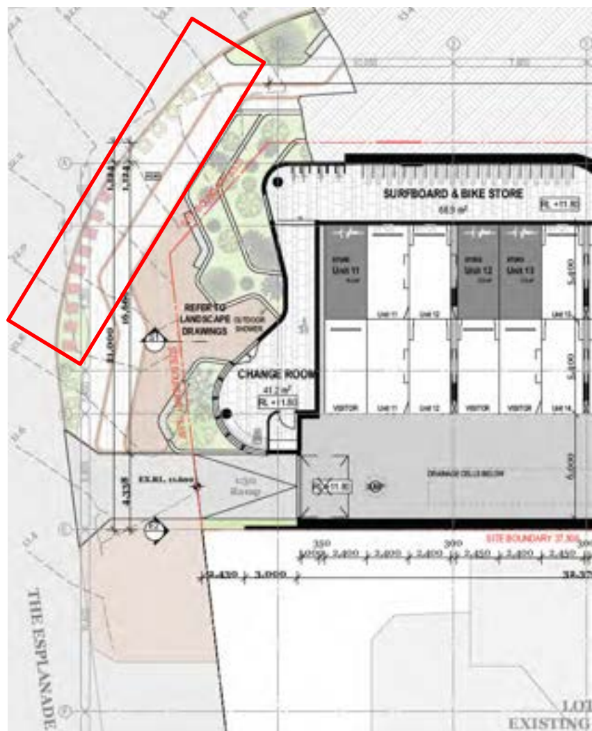
Figure 4-4 On-Street Waste Collection Hardstand
