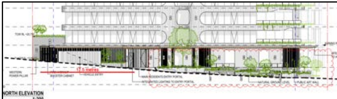
Figure 10: The Brighton Road elevation of the podium, with the garage structure annotated.
