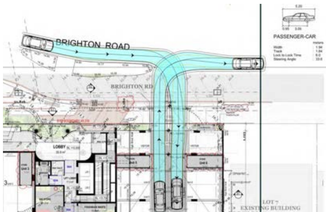
Figure 2-1 RT In and Out Brighton Road Access
