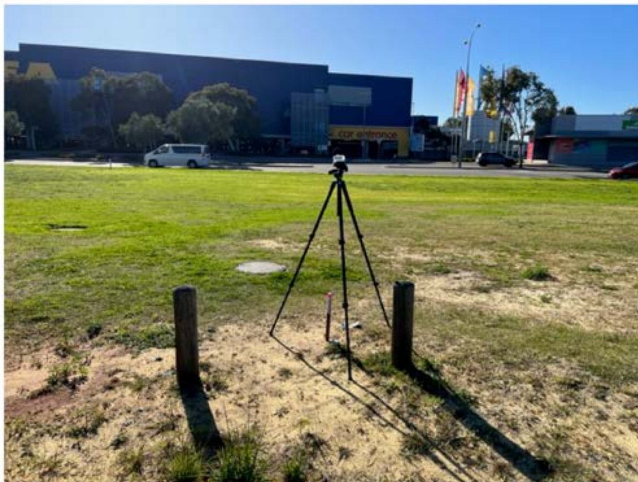
Figure 3-1: Photograph of Sound Level Meter on Site
