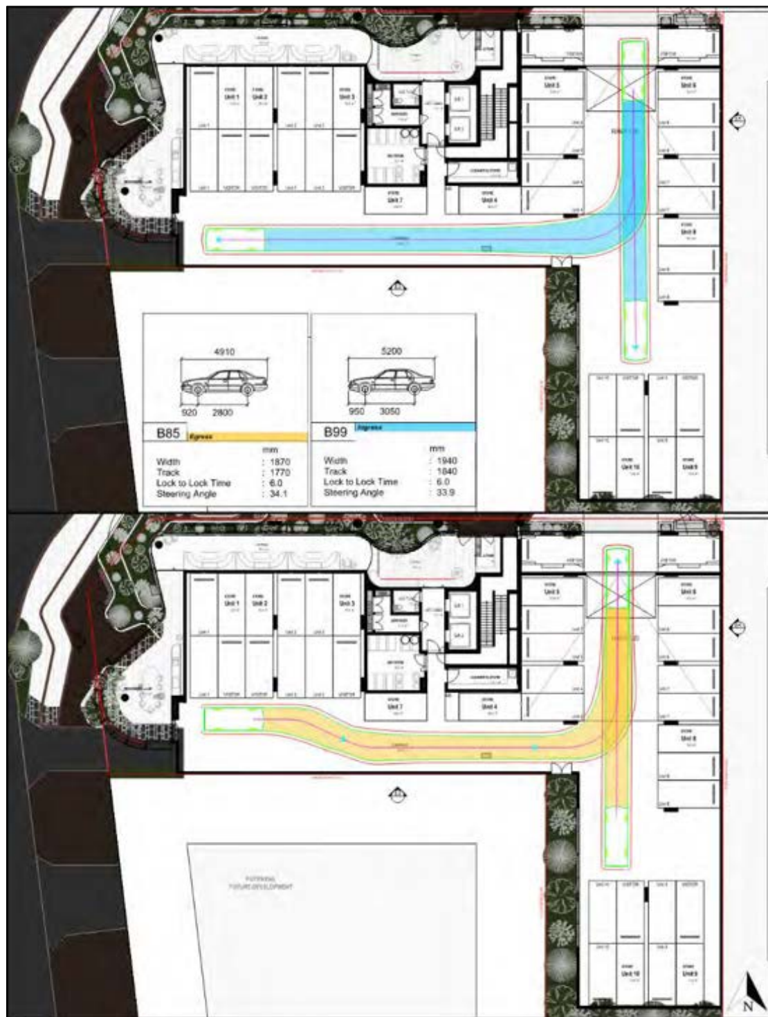
Figure 5-4 Swept Paths – Circulation on the Ground Floor
