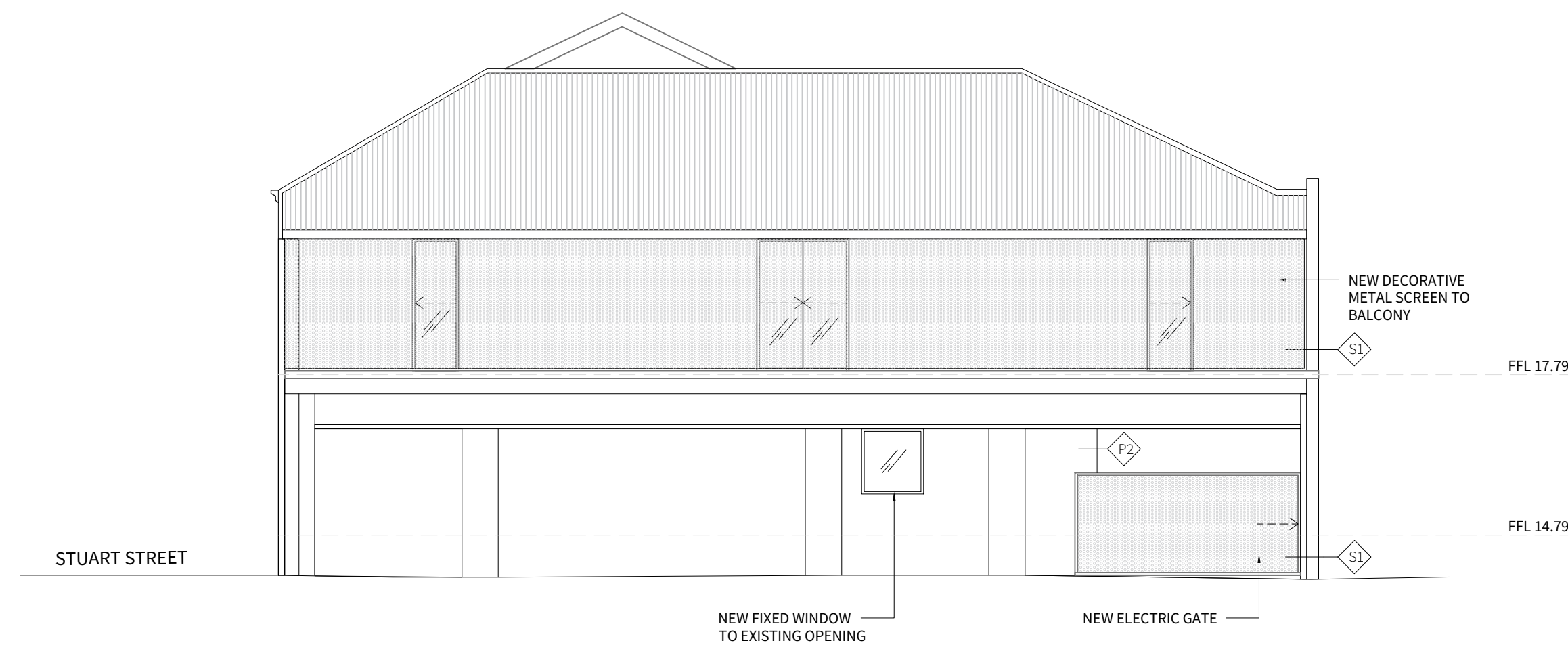
PROPOSED NORTH WEST ELEVATION
