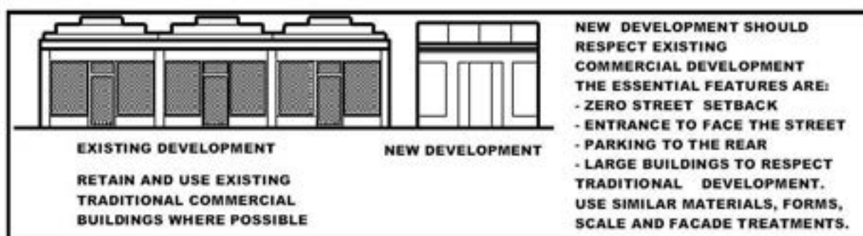
Figure 17 – Example of New and Existing Development
