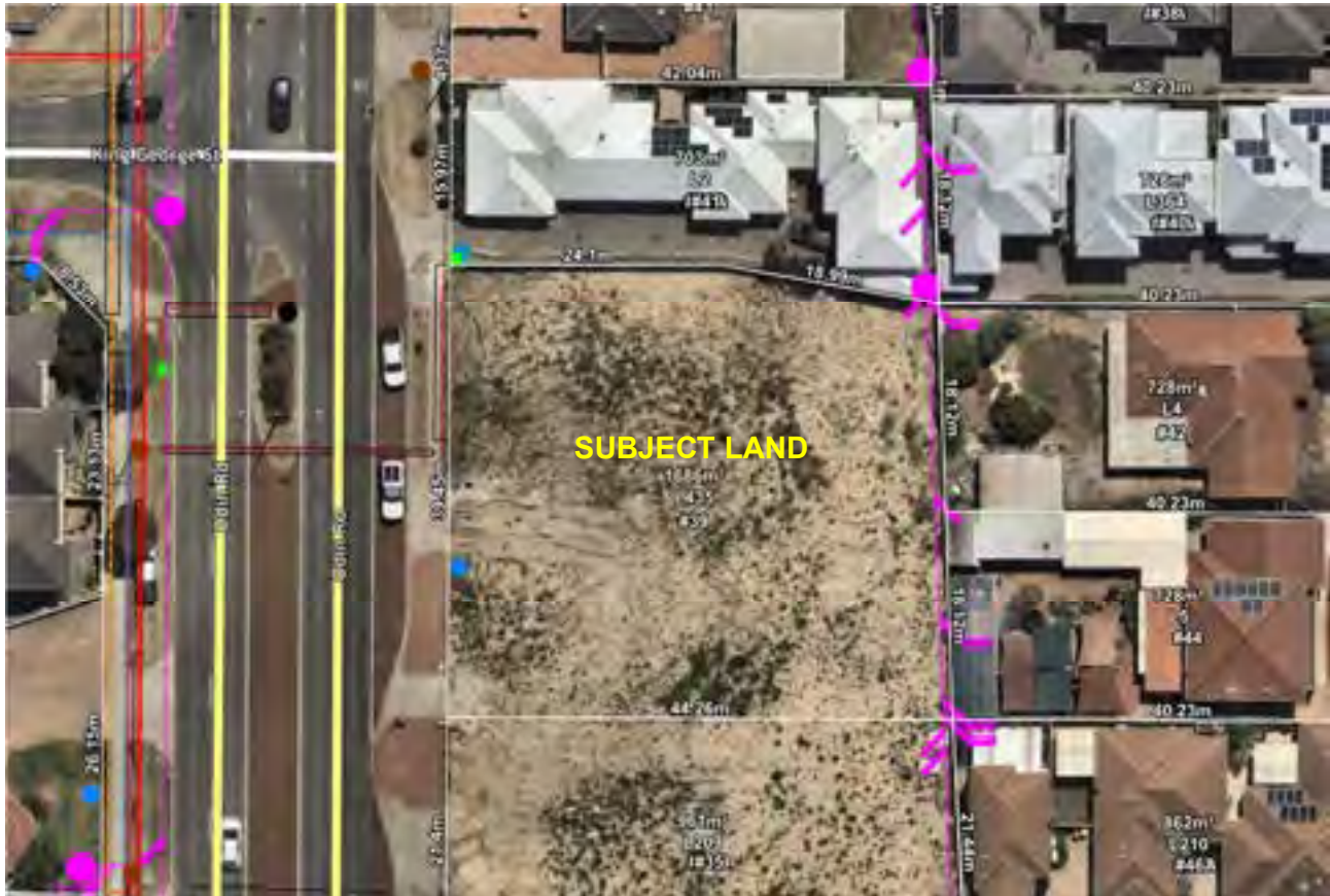
Figure 5 – The existing services in and around the subject land. Services include water, sewerage, electricity and telecommunications. The site is also well serviced with a pedestrian path network that provides good connection with the surrounding area (MNG Mapping).
