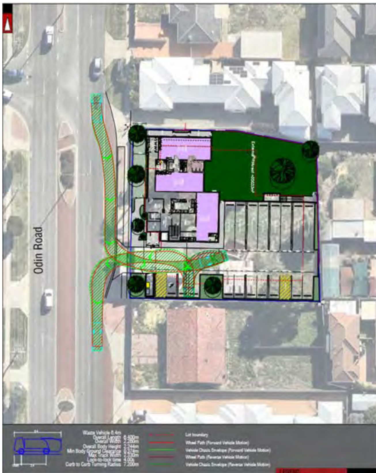
Figure 3 – On-site turning area for the waste collection truck (KCTT)
