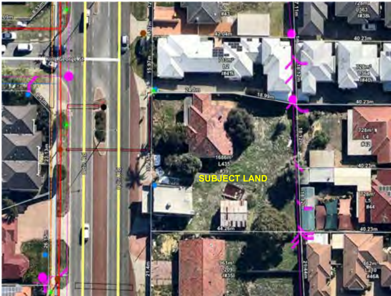
Figure 5 – The existing services in and around the subject land. Services include water, sewerage, electricity and telecommunications. The site is also well serviced with a pedestrian path network that provides good connection with the surrounding area (MNG Mapping).
